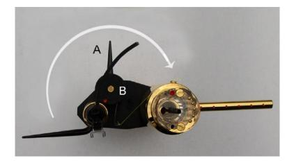
If the handle A is turned in the direction of the arrow the antiskating will increase - and decrease if it is turned the opposite way. If the handle can't be turned enough to get more antiskating, the screw B
